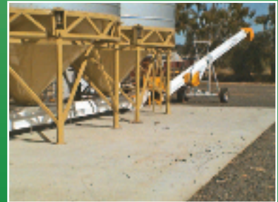
9" undersilo conveyor system stainless
